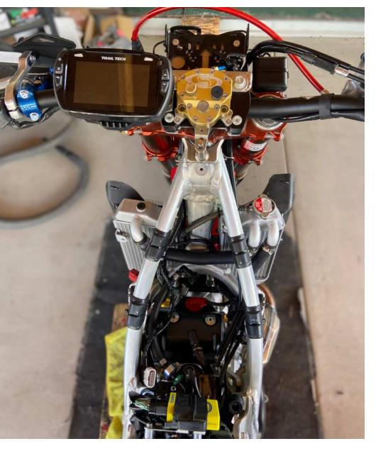
GALFER USA STEEL BRAIDED BRAKE LINE IS USED, ALONG WITH CHAMP ADV CUSTOM STELLA MOUNT, SCOTT'S STEERING STABILIZER, WORKS CONNECTION 123 CLUTCH PERCH SYSTEM, ACERBIS HAND GAURDS, AND A TRAIL TECH COMPUTER
