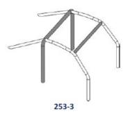
The vertical part of the main rollbar must be as close as possible to the interior contour of the bodyshell and must have only one bend with its lower vertical part. The front pillar of a front rollbar or of a lateral rollbar must follow the windscreen pillars as closely as possible and have only one bend with its lower vertical part.
