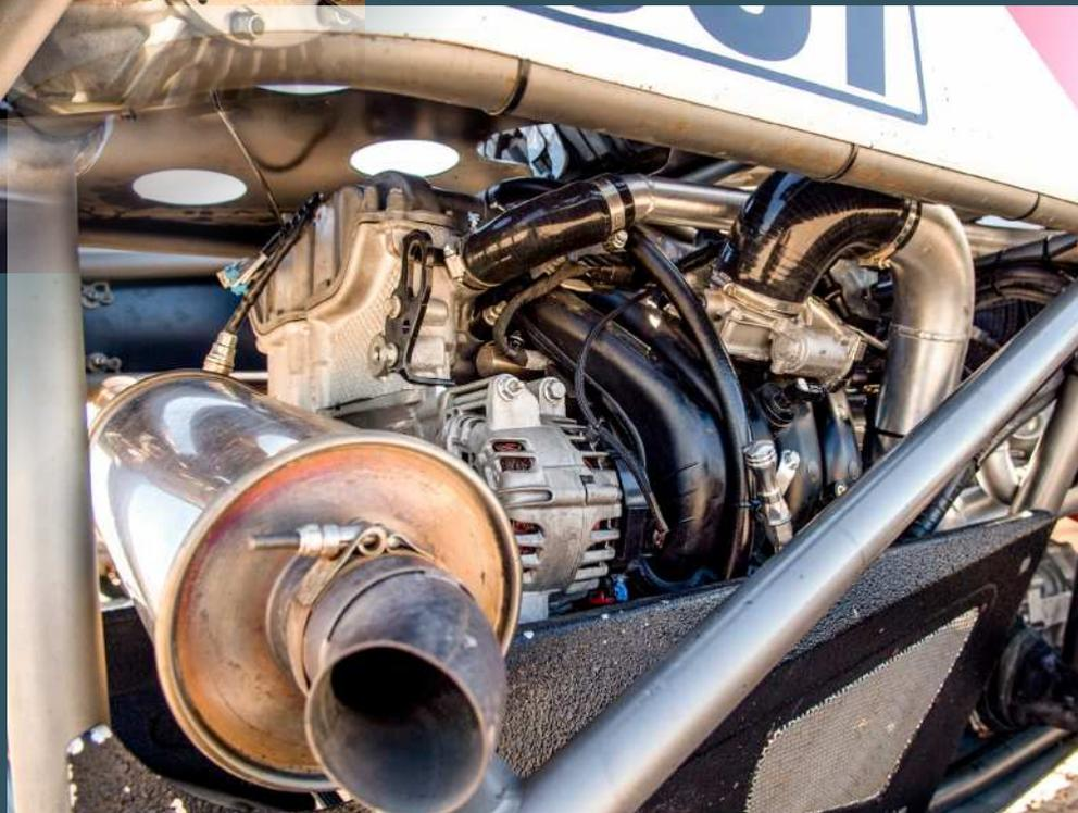
THE NEW CAR IS A CURRY RACE CAR CHASSIS THAT WAS CAD DESIGNED AND MADE FROM 4130 CHROMOLY
