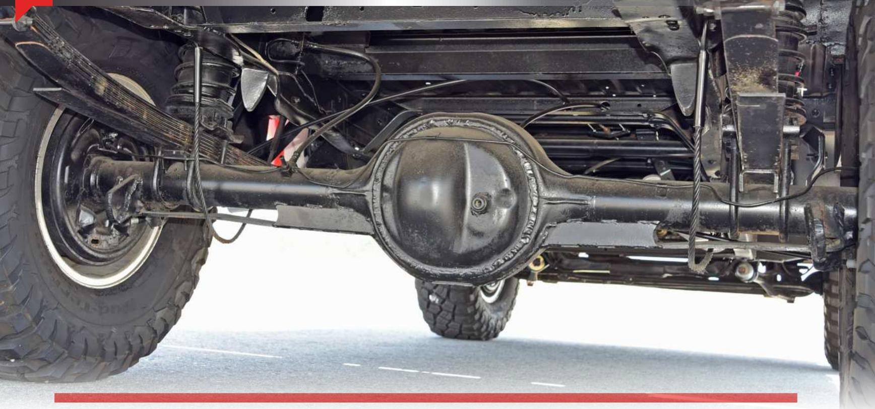
**THE REAR AXLE WAS TRUSSED TO HELP KEEP IT STRAIGHT WHILE GETTING BASHED ACROSS HUNDREDS OF MILES OF DESERT RACING. YOU CAN ALSO SEE THE PRIMITIVE, YET EFFECTIVE LIMITING STRAPS MADE FROM LOOPS OF STEEL CABLE.**
