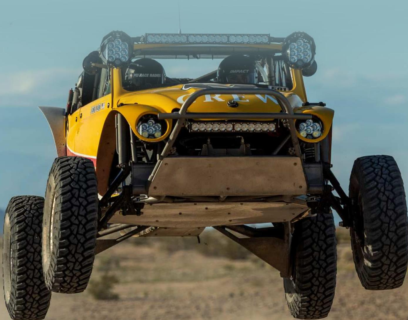
**THE FRONT OF THE NEW CAR FEATURES PROAM CV JOINTS WITH FODRILL KING KONG ARMS AND SPINDLES CONTROLLED BY FOX 12-INCH 2.0 COIL-OVERS**
